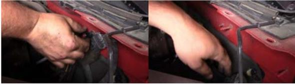
17. Remove the wire connector nut, wire connector, and the loom bracket.
