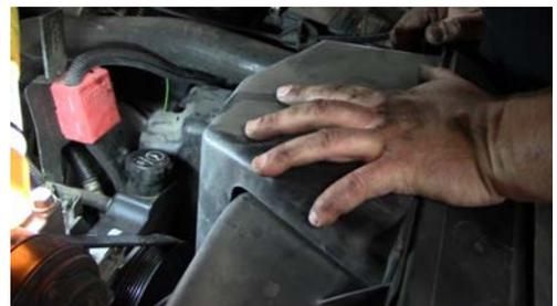
15. Snap the TCM back into the TCM cover and reinstall the cover using the two bolts.
