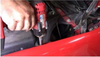
16. Up at the fire wall remove the fender brace.
