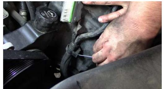
4. Release the clip holding the wires on the ECM cover. Push the wires to the side.
