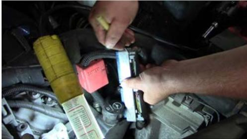
7. Remove the gray plastic backing by releasing the tabs with a small screw driver.
