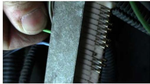
11. Using the supplied wire, feed the end with the pin into terminal 71. Push the pin until the plastic release snaps in place.
