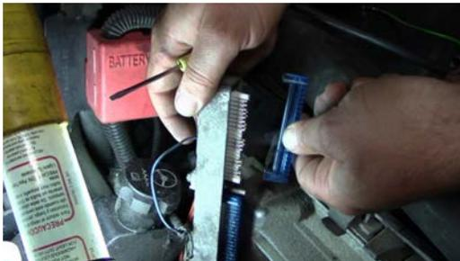
9. Locate the blue shield on the opposite side of terminal 71. Remove it by releasing the plastic tabs
