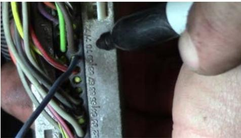
8. On the now exposed connector, locate terminal 71. It will be an empty pocket.
