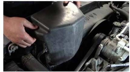
1. Remove the two bolts holding the TCM cover on and lift up the cover.
