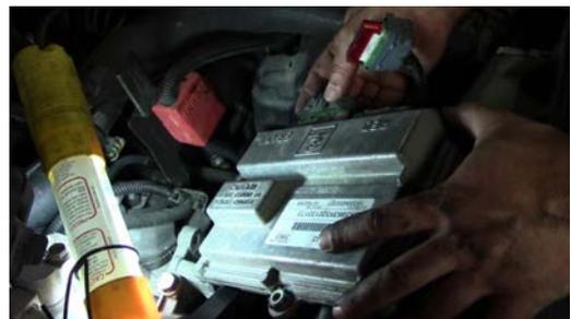
14. Clip the wires back into the ECM cover. Plug the connectors back into the TCM. Note the color of the connectors match the labels on the TCM.
