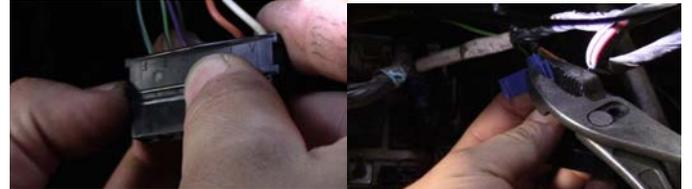
23. Locate the terminal with a letter F. It is on the end. Using the supplied Scotch Lock connector and a pair of pliers, attach the High Idle wire to the brake switch wire.
