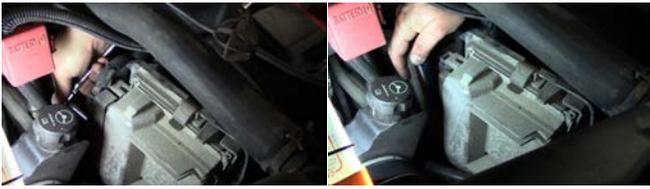
6. Use a 7mm socket to pull off the ECM connector closest to the power steering pump.
