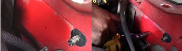
19. Locate the dimple in the firewall. Drill a hole at the dimple to fit the supplied grommet. Deburr hole. Install grommet.
