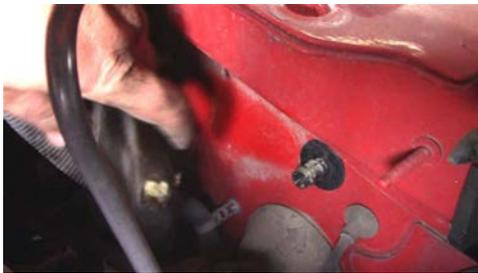
18. Remove the clip and pull back the fire wall insulation.
