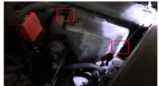
5. Release the two locking tabs on the ECM cover. Pull up the ECM cover and set aside. The ECM is now exposed. You do not need to pull the ECM out for this job.
