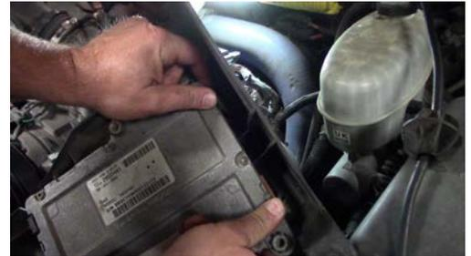
2. Release the tabs holding the TCM into the cover. Set cover aside.
